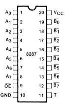
Figure 2. 8287 Pin Configuration
